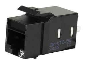
Category 5e Keystone jack, 8-position, 180 degree exit, icon compatible, T568A/B wiring, Black, individually packaged. Keystone, KT2J jacks and modules feature New installer friendly lacing cap termination with free termination tool in every carton. The keystone footprint allows flexibility in installation scheduling because its rear insertion into the faceplate allows the technician to complete the termination before and during the construction process.
