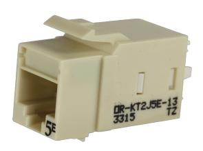
Category 5e Keystone jack, 8-position, 180 degree exit, icon compatible, T568A/B wiring, Elec Ivory, individually packaged. Keystone, KT2J jacks and modules feature New installer friendly lacing cap termination with free termination tool in every carton. The keystone footprint allows flexibility in installation scheduling because its rear insertion into the faceplate allows the technician to complete the termination before and during the construction process.
