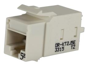
Category 5e Keystone jack, 8-position, 180 degree exit, icon compatible, T568A/B wiring, Fog White , individually packaged.Keystone, KT2J jacks and modules feature New installer friendly lacing cap termination with free termination tool in every carton. The keystone footprint allows flexibility in installation scheduling because its rear insertion into the faceplate allows the technician to complete the termination before and during the construction process.
