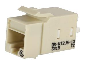
Category 6 Keystone jack, 8-position, 180 degree exit, icon compatible, T568A/B wiring, Elec Ivory, individually packaged. Keystone, KT2J jacks and modules feature New installer friendly lacing cap termination with free termination tool in every carton. The keystone footprint allows flexibility in installation scheduling because its rear insertion into the faceplate allows the technician to complete the termination before and during the construction process.
