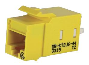
Category 6 Keystone jack, 8-position, 180 degree exit, icon compatible, T568A/B wiring, Yellow, individually packaged. Keystone, KT2J jacks and modules feature New installer friendly lacing cap termination with free termination tool in every carton. The keystone footprint allows flexibility in installation scheduling because its rear insertion into the faceplate allows the technician to complete the termination before and during the construction process.
