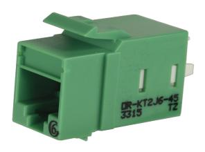
Category 6 Keystone jack, 8-position, 180 degree exit, icon compatible, T568A/B wiring, Green , individually packaged. Keystone, KT2J jacks and modules feature New installer friendly lacing cap termination with free termination tool in every carton. The keystone footprint allows flexibility in installation scheduling because its rear insertion into the faceplate allows the technician to complete the termination before and during the construction process.
