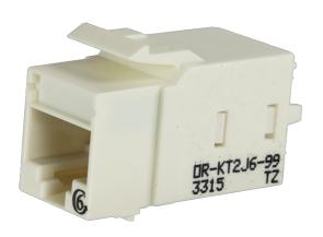
Category 6 Keystone jack, 8-position, 180 degree exit, icon compatible, T568A/B wiring, Wiremold Ivory, individually packaged. Keystone, KT2J jacks and modules feature New installer friendly lacing cap termination with free termination tool in every carton. The keystone footprint allows flexibility in installation scheduling because its rear insertion into the faceplate allows the technician to complete the termination before and during the construction process.
