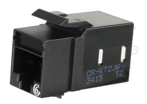
Resealable package of 25 Category 6 Keystone jack, 8-position, 180 degree exit, icon compatible, T568A/B wiring, Black. Keystone, KT2J jacks and modules feature New installer friendly lacing cap termination with free termination tool in every carton. The keystone footprint allows flexibility in installation scheduling because its rear insertion into the faceplate allows the technician to complete the termination before and during the construction process.
