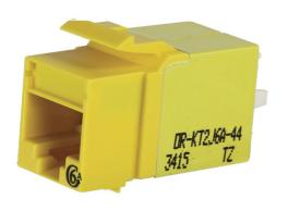
Category 6A Keystone jack, 8-position, 180 degree exit, icon compatible, T568A/B wiring, Yellow, individually packaged. Keystone, KT2J jacks and modules feature New installer friendly lacing cap termination with free termination tool in every carton. The keystone footprint allows flexibility in installation scheduling because its rear insertion into the faceplate allows the technician to complete the termination before and during the construction process.
