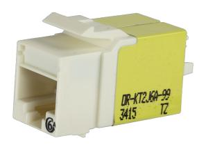
Category 6A Keystone jack, 8-position, 180 degree exit, icon compatible, T568A/B wiring, Wiremold Ivory, individually packaged. Keystone, KT2J jacks and modules feature New installer friendly lacing cap termination with free termination tool in every carton. The keystone footprint allows flexibility in installation scheduling because its rear insertion into the faceplate allows the technician to complete the termination before and during the construction process.
