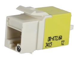
Category 6A Keystone jack, 8-position, 180 degree exit, icon compatible, T568A/B wiring, Fog White, individually packaged. Keystone, KT2J jacks and modules feature New installer friendly lacing cap termination with free termination tool in every carton. The keystone footprint allows flexibility in installation scheduling because its rear insertion into the faceplate allows the technician to complete the termination before and during the construction process.
