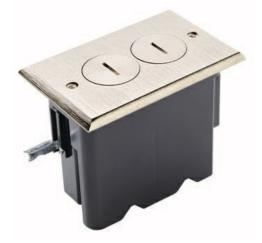
A rectangular wood floor box kit with a nickel finish that supplies power in open space living. The kit includes the box, cover and a 15A Tamper resistant receptacle. It can be installed on carpet, wood, natural stone and tile floors that have a wooden subfloor.
