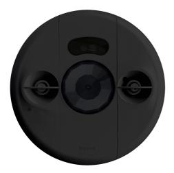
The LMDC-100 low profile Dual Technology Ceiling Mount Occupancy Sensor uses both passive infrared (PIR) and ultrasonic technologies to achieve precise occupancy sensing for energyefficient control of lighting and plug loads. It is a digital sensor, and is part of a Wattstopper Digital Lighting Management (DLM) system.
