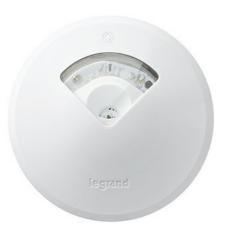
The LMDL-600 is a wireless open loop photo sensor that measures the daylight contribution in order to automatically switch or dim multiple zones of lighting. It is part of the NEW wireless Digital Lighting Management (DLM) system and sends light level signals to control loads connected to DLM on/off or dimming room controllers.
