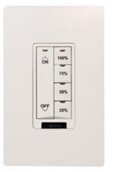
The LMDM-101 Digital Dimming Wall Switch is a low voltage device for dimming control of one or more lighting loads. It is part of a Digital Lighting Management (DLM) system and can dim load(s) connected to DLM dimming room controllers and switch load(s) connected to DLM on/off room controllers.
