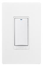
The LMDM-601 Dimming Wall Switch is a wireless low voltage device for dimming control of one or more lighting loads. It is part of the wireless Digital Lighting Management (DLM) system and can dim load(s) connected to wireless DLM dimming room controllers (LMRC-611) for a totally wireless room. Alternatively it can be used in a hybrid wired & wireless room to control loads connected to a traditional wired room controller (e.g. LMRC-111) when used in conjunction with a wireless bridge (LMBC-650).
