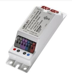
The LMFC-011 fixture controller mounts in individual lighting fixtures to give them connectivity to a Digital Lighting Management (DLM) system. The controller provides a 0-10 volt signal for control of dimmable loads including compatible LED drivers and electronic ballasts and connects to the DLM local network via a single- or dual-port RJ45 wiring whip (ordered separately). Each DLM local network can support up to 64 loads.
