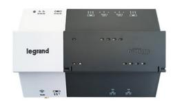
The LMJA-8xxx-AX (using AX 3.8) is a network controller designed to communicate with wired and wireless DLM network Bridges, for local in-room wired networks and/or LMCP panels. It provides control, monitoring, adjustment, and standard or Human Centric Lighting (HCL) scheduling functionality for networked DLM systems. The Network Supervisor is a PC server running similar software designed to coordinate control of multiple LMJA-8xxx's and store historical data.
