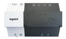
The LMJA-8xxx-SM is a Network Controller designed to communicate with Wired and Wireless DLM Network Bridges, for local in-room wired networks and/or LMCP panels. It provides control, monitoring, adjustment, and standard or Human Centric Lighting (HCL) scheduling functionality for networked DLM systems. The Network Supervisor is a PC server running similar software designed to coordinate control of multiple LMJA-8xxx-SMs and store historical data.
