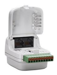
The LMOR-102 is an accessory interface device with two low voltage mechanically held relays. Other components of a Wattstopper Digital Lighting Management (DLM) System can control the relays similar to the line voltage relays in a room controller. This allows the two dry output contacts to control products that provide a 0-24V AC/DC input signal.
