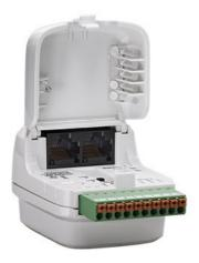
The LMOR-102 is an accessory interface device with two low voltage mechanically held relays. Other components of a Wattstopper Digital Lighting Management (DLM) System can control the relays similar to the line voltage relays in a room controller. This allows the two dry output contacts to control products that provide a 0-24V AC/DC input signal.
