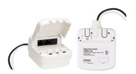
The LMPB-100 Digital Power Booster includes a high-efficiency switching power supply to add power to a DLM local network. It can be used with LMFC fixture controllers or any other Wattstopper Digital Lighting Management (DLM) controllers to allow integration of occupancy sensors, daylighting sensors and switches for energy-efficient lighting control. This device does not include a relay for load control
