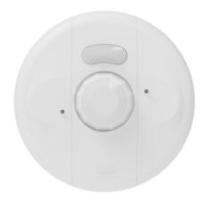
The LMPC-100 low profile Digital PIR Ceiling Mount Occupancy Sensor uses passive infrared (PIR) technology and one of three lenses to detect occupancy in different types of spaces for energyefficient control of lighting and plug loads. It is a digital sensor, and is part of a Wattstopper Digital Lighting Management (DLM) system.
