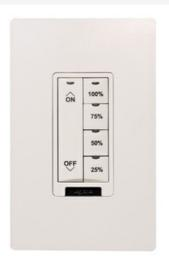
The LMPS-104 Digital Partition Switch enables quick manual coordination of lighting controls in flexible spaces with up to four movable walls. It is part of a Digital Lighting Management (DLM) system, and can reconfigure connected switches and occupancy sensors. The LMPS-104 may also be used as a status indicator when an LMIO-102 Digital Partition Interface is used for automatic coordination of controls.
