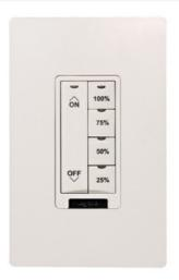
The LMPS-104 Digital Partition Switch enables guick manual coordination of lighting controls in flexible spaces with up to four movable walls. It is part of a Digital Lighting Management (DLM) system, and can reconfigure connected switches and occupancy sensors. The LMPS-104 may also be used as a status indicator when an LMIO-102 Digital Partition Interface is used for automatic coordination of controls.
