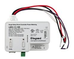
LMRC-111-16M room controllers include one relay capable of switching a 16 amp load, a high-efficiency intelligent switching power supply and both Class 1 and Class 2 0-10 volt outputs for control of dimmable loads including compatible LED drivers or electronic ballasts. Room Controllers are the foundation of a Digital Lighting Management (DLM) system, and allow integration of occupancy sensors, daylighting controls and switches for energyefficient control.
