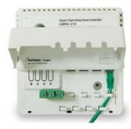
LMRC-210 Series Digital Room Controllers include one, two or three relay(s) to switch a total of 15 or 20 amps, a highefficiency switching power supply and one 0-10 volt output per relay for control of dimmable loads including electronic ballasts (Advance Mark 7, or equivalent). They are the foundation of a Wattstopper Digital Lighting Management (DLM) system, and allow integration of occupancy sensors, daylighting controls and switches for energy-efficient lighting control.
