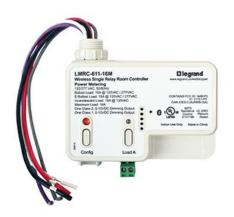
The LMRC-611-16M is a wireless DLM room controller, part of the foundation of the wireless Digital Lighting Management (DLM) system which includes occupancy sensors, daylighting controls, and switches for energy-efficient control. The LMRC-611-16M includes one relay to switch a total of 16 amps, a high-efficiency switching power supply, and both Class 1 and Class 2 0–10 volt outputs for control of dimmable loads including compatible LED drivers and electronic ballasts.
