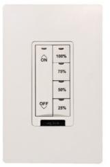
LMSW-100 Series Digital Wall Switches are low voltage devices for energysaving manual on/ off control of one or more loads from one or more locations. They are part of a Digital Lighting Management (DLM) system and can control any load(s) connected to DLM room controllers.
