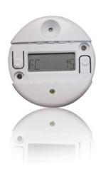
The LS-102 Daylighting Controller is a single zone, on/off switching device designed to be installed in a closed loop application. A self-contained 24 VDC device with an extended range of 1-1400 footcandles, the LS-102 requires a low voltage power pack to operate. The controller consists of an advanced digital multi-band photosensor, an on-board microcontroller, and an LCD display. This photosensor is positioned behind a 100° cone that cuts off unwanted light, preventing false triggers.
