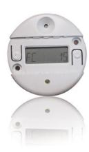
The LS-102 Daylighting Controller is a single zone, on/off switching device designed to be installed in a closed loop application. A self-contained 24 VDC device with an extended range of 1-1400 footcandles, the LS-102 requires a low voltage power pack to operate. The controller consists of an advanced digital multi-band photosensor, an on-board microcontroller, and an LCD display. This photosensor is positioned behind a 100° cone that cuts off unwanted light, preventing false triggers.
