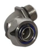
Rated IP68 and NEMA 4X, Stainless Steel Liquid-Tight Connectors offer corrosion resistance for the toughest environments. For use in wet or dry locations to seal electrical connections against dust, dirt, oil, water, chemicals and other corrosive elements. These are available in straight and 90 degree, 3/8"" to 2"" NPT. The stainless steel liquid-tight offering includes a nylon-insulated throat and Viton 0-Ring.
