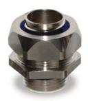
Rated IP68 and NEMA 4X, Stainless Steel Liquid-Tight Connectors offer corrosion resistance for the toughest environments. For use in wet or dry locations to seal electrical connections against dust, dirt, oil, water, chemicals and other corrosive elements. These are available in straight and 90 degree, 3/8"" to 2"" NPT. The stainless steel liquid-tight offering includes a nylon-insulated throat and Viton 0-Ring.
