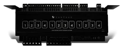
The Low-Voltage Output Station (LVOS) is used for the control and automation of LED, CFL, and CCFL lighting loads requiring either 0-10 or pulse width modulation (PWM) for dimming control. The dry contact inputs can be used with motion sensors, light sensors, pressure sensors, IR inputs, magnetic switches, and more. As part of the Legrand lighting solution, it provides control of LED loads as well as inputs from dry contacts for lighting and automation.
