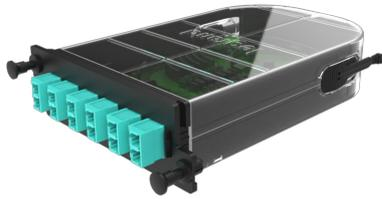
Infinium M4 SC Splice Cassettes enable industry leading performance, fast field termination, and provide cable management within the housing. The Splice Cassettes are designed for use with Single-Mode (OS2) or Multimode (OM4/OM5) Fiber, Houses 12-24. Compatible with Infinium HD-E Rack Mount Fiber Enclosure with M4 Drawer Face.
