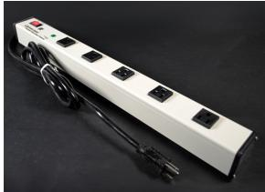
Perma Power computer grade surge protection. Five outlets, lighted switch, durable putty white aluminum housing, 15A. Receptacles rotated 90 degrees and spaced to accommodate transformers. 6' (1.8m) 14/3 SJT putty white cord with NEMA5-15 plug. Length 13 1/4"" (337mm). Snap-on, slide-off mounting.
