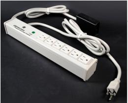
Perma Power computer grade surge protection. Six outlets, remote switch, durable putty white aluminum housing, 15A. 6' (1.8m) 14/3 SJT putty white cord with NEMA5-15 plug. Length 13 1/4"" (337mm). Snap-on, slide-off mounting.
