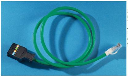
Clarity 6 Patch Cord, Category 6, modular 8-position to 110. Cord is terminated on one end with a male 110 plug with internal signal feedback technology, which reduces crosstalk without compromising impedance. The other cord end is terminated with an 8-position modular plug with Ortronics Paralign 2 pair isolation technology.
