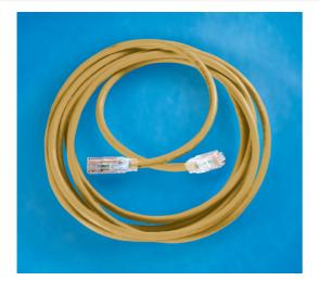
Clarity 5E Premium Category 5e Modular Patch Cord, yellow, 3', Category 5e, four-pair UTP stranded 24 AWG PVC/CM, center tuned with Clarity 5E connecting hardware for optimum Category 5e installed performance using Ortronics Paralign 2 pair-positioning technology
