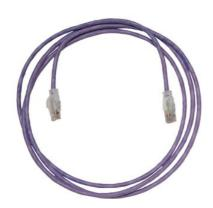
Clarity 5E Premium Category 5e Modular Patch Cord, purple, 3', Category 5e, four-pair UTP stranded 24 AWG PVC/CM, center tuned with Clarity 5E connecting hardware for optimum Category 5e installed performance using Ortronics Paralign 2 pair-positioning technology
