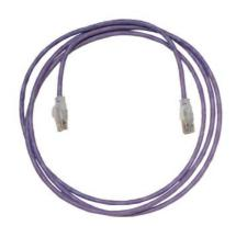
Clarity 5E Premium Category 5e Modular Patch Cord, purple, 3', Category 5e, four-pair UTP stranded 24 AWG PVC/CM, center tuned with Clarity 5E connecting hardware for optimum Category 5e installed performance using Ortronics Paralign 2 pair-positioning technology
