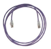
Clarity 5E Premium Category 5e Modular Patch Cord, purple, 5', Category 5e, four-pair UTP stranded 24 AWG PVC/CM, center tuned with Clarity 5E connecting hardware for optimum Category 5e installed performance using Ortronics Paralign 2 pair-positioning technology
