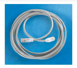
Clarity 5E Premium Category 5e Modular Patch Cord, gray, 5', Category 5e, four-pair UTP stranded 24 AWG PVC/CM, center tuned with Clarity 5E connecting hardware for optimum Category 5e installed performance using Ortronics Paralign 2 pair-positioning technology.
