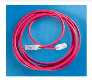
Clarity 5E Premium Category 5e Modular Patch Cord, red, 9', Category 5e, four-pair UTP stranded 24 AWG PVC/CM, center tuned with Clarity 5E connecting hardware for optimum Category 5e installed performance using Ortronics Paralign 2 pair-positioning technology.
