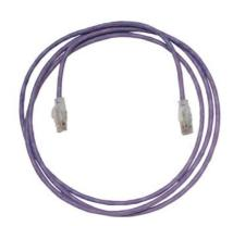
Clarity 5E Premium Category 5e Modular Patch Cord, purple, 15', Category 5e, four-pair UTP stranded 24 AWG PVC/CM, center tuned with Clarity 5E connecting hardware for optimum Category 5e installed performance using Ortronics Paralign 2 pair-positioning technology
