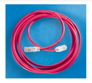
Clarity 6 Modular Patch Cord, red 3', Category 6, four-pair UTP stranded 24 AWG PVC/CM, center tuned with Clarity 6 connecting hardware for optimum Category 6 installed performance using Ortronics Paralign 2 pair-positioning technology
