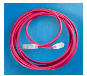
Clarity 6 Modular Patch Cord, red, 5', Category 6, four-pair UTP stranded 24 AWG PVC/CM, center tuned with Clarity 6 connecting hardware for optimum Category 6 installed performance using Ortronics Paralign 2 pair-positioning technology
