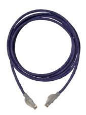
Clarity 6 Modular Patch Cord, purple, 5', Category 6, four-pair UTP stranded 24 AWG PVC/CM, center tuned with Clarity 6 connecting hardware for optimum Category 6 installed performance using Ortronics Paralign 2 pair-positioning technology
