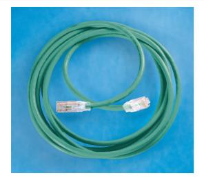
Clarity 6 Modular Patch Cord, green, 7', Category 6, four-pair UTP stranded 24 AWG PVC/CM, center tuned with Clarity 6 connecting hardware for optimum Category 6 installed performance using Ortronics Paralign 2 pair-positioning technology
