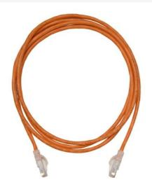
Clarity 6 Modular Patch Cord, orange, 9', Category 6, four-pair UTP stranded 24 AWG PVC/CM, center tuned with Clarity 6 connecting hardware for optimum Category 6 installed performance using Ortronics Paralign 2 pair-positioning technology
