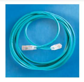
Clarity 6 Modular Patch Cord, blue, 10', Category 6, four-pair UTP stranded 24 AWG PVC/CM, center tuned with Clarity 6 connecting hardware for optimum Category 6 installed performance using Ortronics Paralign 2 pair-positioning technolgy
